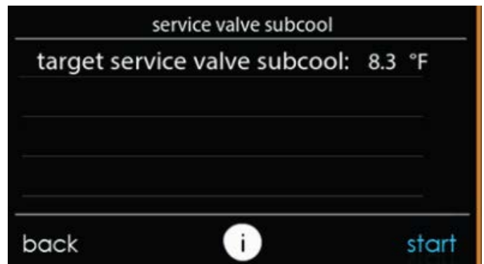
Fig. 16 – Liquid Service Valve Subcooling Target
