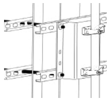
I-Beam (Column) Installation
