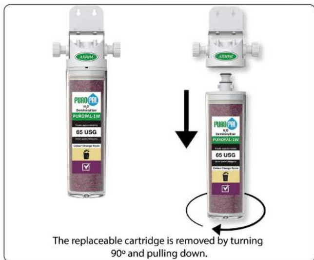
Figure 2 - Replacing cartridge
