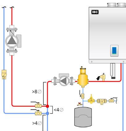
① Closely-spaced tees: install tees with straight piping (min. pipe diameter lengths as shown), with tees maximum 4 pipe diameters apart with no restrictions between fittings
