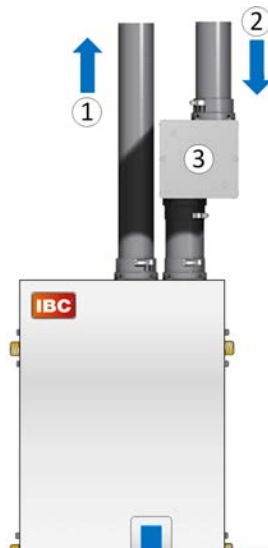
Figure 31 Direct vent - intake, exhaust system with optional air intake filter (filtration may also be used on indoor air applications as required)
