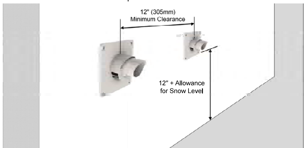
Figure 21: Horizontal Polypropylene Concentric Termination - Two Kits
