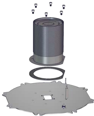
Figure 75 Removing bolts securing burner to heat exchanger lid
