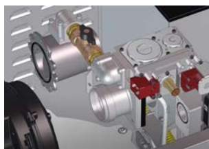
Figure 72 Removing mixer assembly, gas line and gas valve
