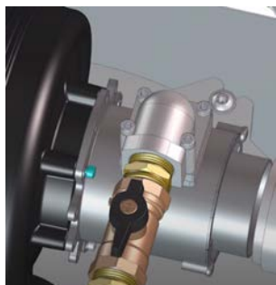
Figure 71 Removing bolts securing mixer to fan
