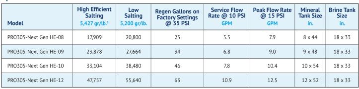
System conforms to NSF/ANSI44 for specific performance claims. Efficiency is measured by laboratory test described in NSF/ANSI44.
