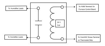
Fig. 38 – Field-supplied Isolation Relay for Humidifiers with
