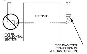
Fig. 51 – Combustion Air and Vent Pipe Diameter Transition
