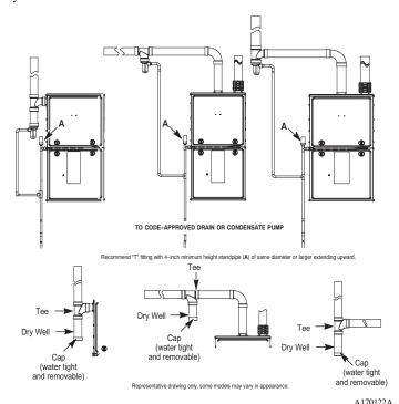
Fig. 52 – Recommended Combustion Air Inlet Moisture Trap
