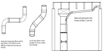
Fig. 53 – Near Furnace Vent Connections
