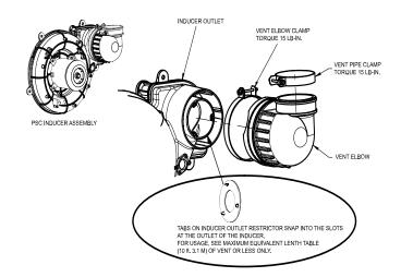
Fig. 54 - Inducer Vent Elbow
