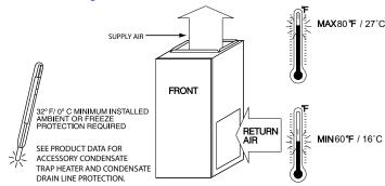
Fig. 3 – Freeze Protection and Return Air Temperature
