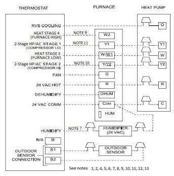
2-Stage Furnace with Heat Pump
