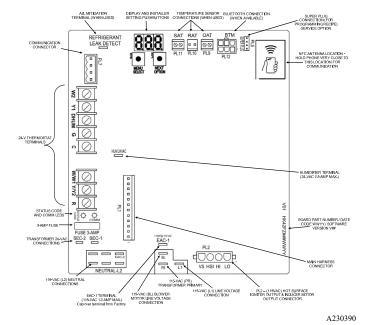
Fig. 39 - Example of Variable Speed Furnace Control
