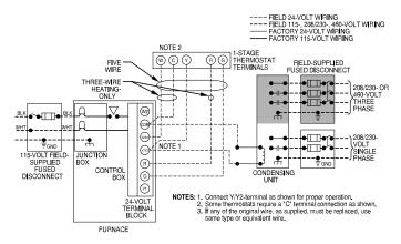
Fig. 34 – Typical Two-Stage Field Wiring Diagram
