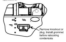
Fig. 18 - Horizontal Drain Trap Grommet
