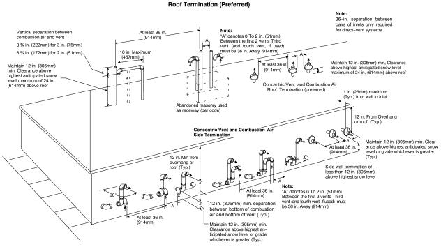
Fig. 41 – Combustion Air and Vent Pipe Termination for Direct Vent (2-Pipe) System
