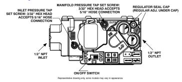
Fig. 65 – Gas Valve with Tower Pressure Ports
