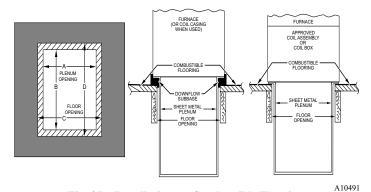
Fig. 25 – Installation on Combustible Flooring
