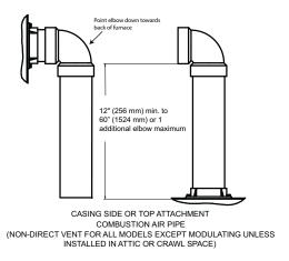
Fig. 48 – Combustion Air Pipe Attachment
