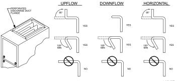
Fig. 20 – Duct Flanges
