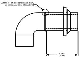
Fig. 17 - Modify Rubber Drain Elbow
