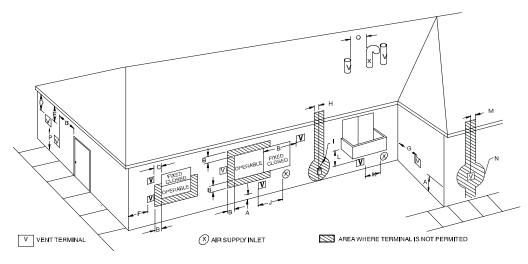
Fig. 44 – Direct Vent Termination Clearance
