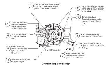
Fig. 9 – Downflow Trap Configuration (Appearance may vary) **Condensate Trap - Horizontal Orientation.**
