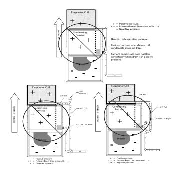
Fig. 13 – Example of Field Drain Attachment (Not Allowed)
