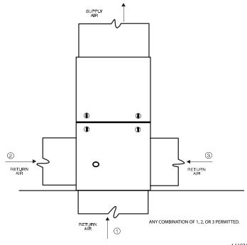
Fig. 21 – Upflow Return Air Configurations and Restrictions
