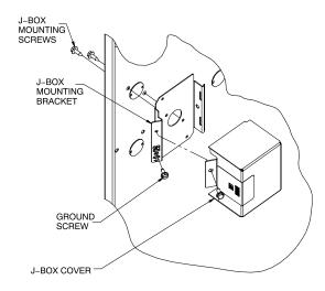
Fig. 35 – Installing J-Box (When Used)
