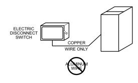
Fig. 33 – Field-Supplied External Electrical Box on Furnace Casing
