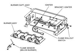
Fig. 68 – Burner Assembly
