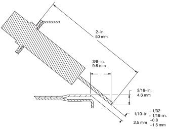
Fig. 70 - Igniter Position - Side View
