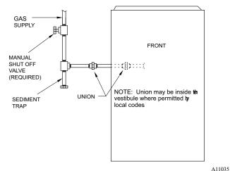
Fig. 32 - Typical Gas Pipe Arrangement
