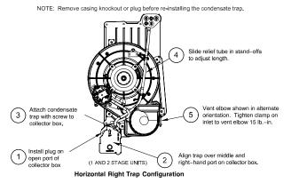
Fig. 10 - Horizontal Right Trap Config (Appearance may vary)
