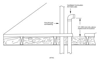
Fig. 49 – Vent Terminations for Ventilated Combustion  $\mathbf{Air}^{\mathrm{A}10497}$
