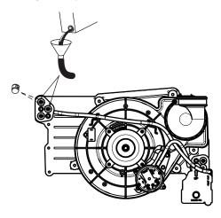
Fig. 63 – Priming Condensate Trap
