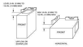
Fig. 19 – Furnace Pitch Requirements
