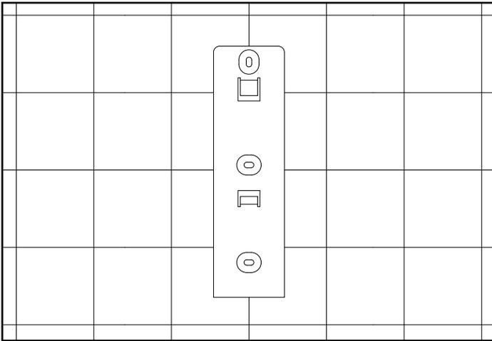
2. Drill the three 6mm or 1/4" holes according to the mounting plate and attach the mounting plate to the wall using the plastic anchors and screws.
