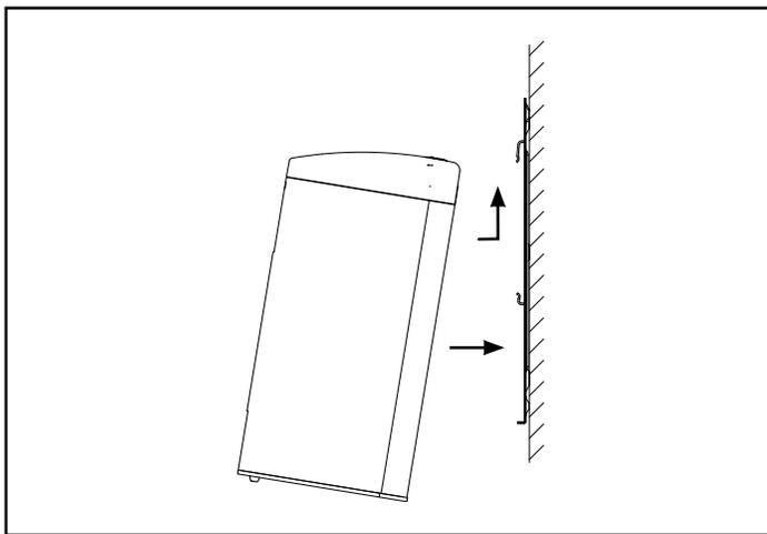
4. Press the dispenser down to attach it to the hook tightly.
