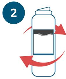
Turn used filter left 1/4 turn to remove from filter head.
