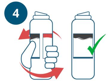
Hold filter as shown above. Firmly insert into filter head. Turn filter 1/4 to the right until it locks into place and the front label is clearly visible.
