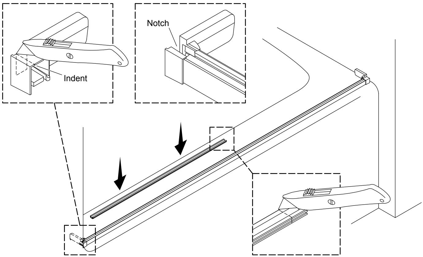
**⚠ CAUTION: Risk of product damage.** A notch is required on the bumper for the fixed panel side only. An indent on the inside top of the bumper indicates where the notch should be cut. **Do not cut a notch in the bumper for the sliding panel side.**
