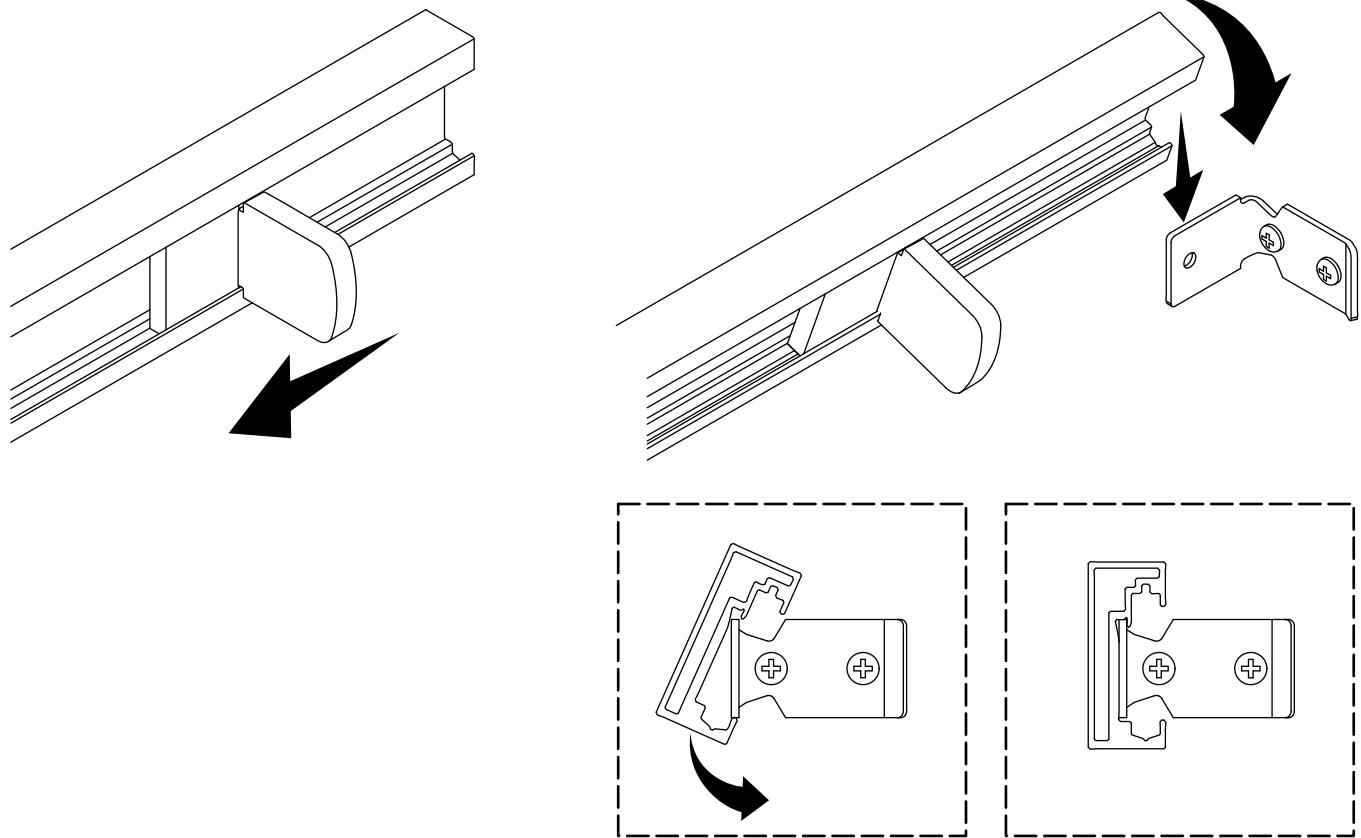
**⚠ CAUTION: Risk of product damage.** The header may fall if not properly positioned onto the wall brackets. Verify that the top of the header is properly hooked onto the brackets.
