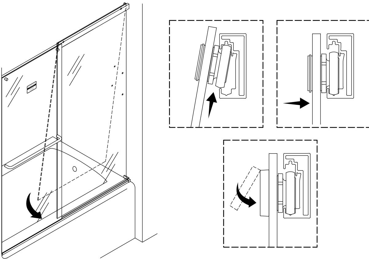
**⚠ CAUTION: Risk of product damage.** Carefully and thoroughly clean the header. Make sure that there is no debris in the roller tracks.
