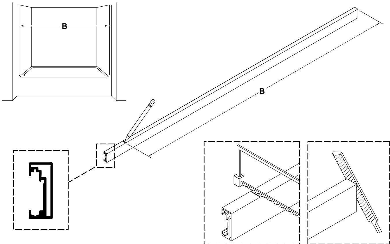
**IMPORTANT!** Confirm your measurements before cutting. Do not cut the header too short.
