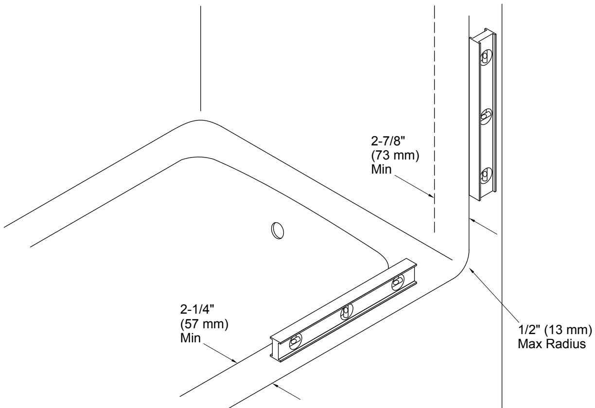
**IMPORTANT!** For proper door alignment and operation, confirm that the shower base/bath ledge and walls meet the following requirements. Do not install the door if these requirements are not met.
