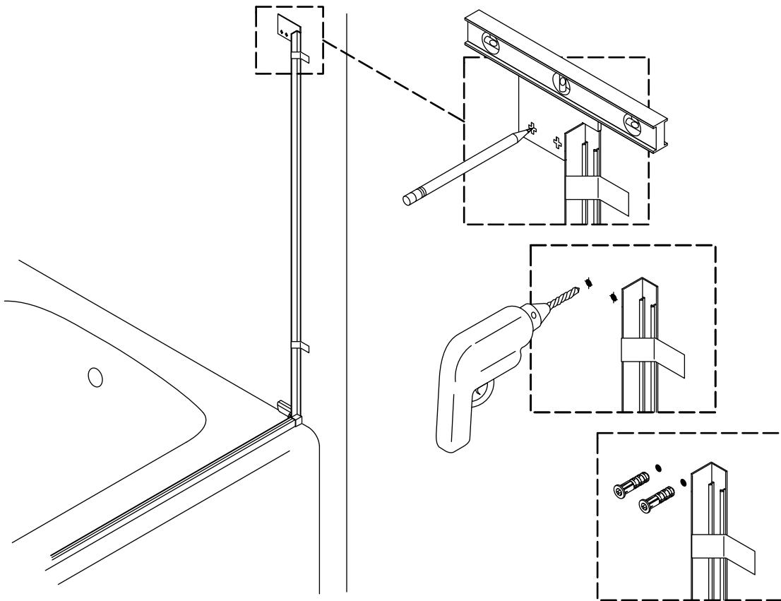
**IMPORTANT!** The wall seal must be level and plumb for proper header installation.
