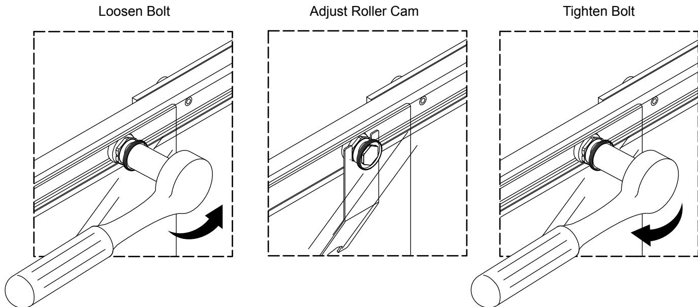
**NOTICE:** The panels may require adjustment to ensure that they touch the top and bottom bumpers in the proper closed position.
