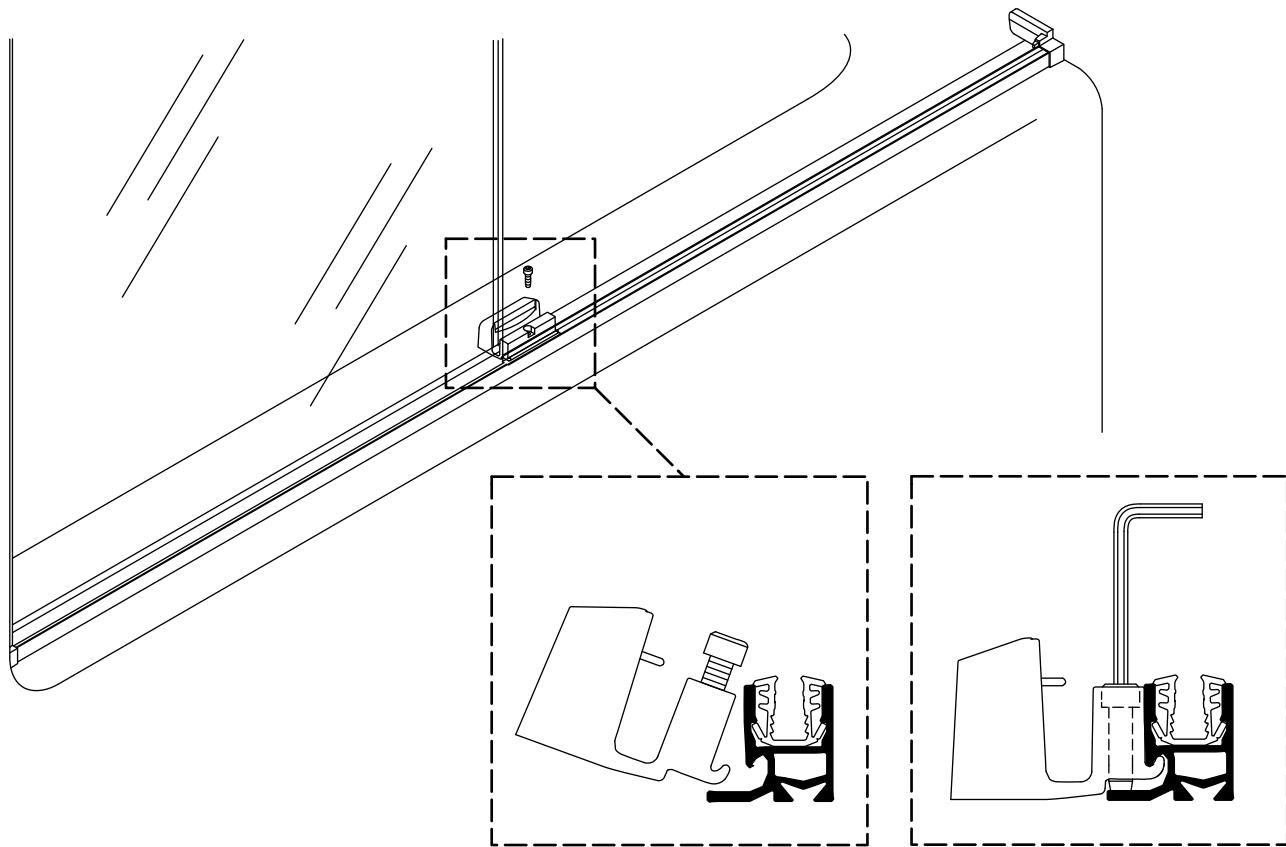
**IMPORTANT!** The centerguide must be fully seated behind the threshold lip as shown.
