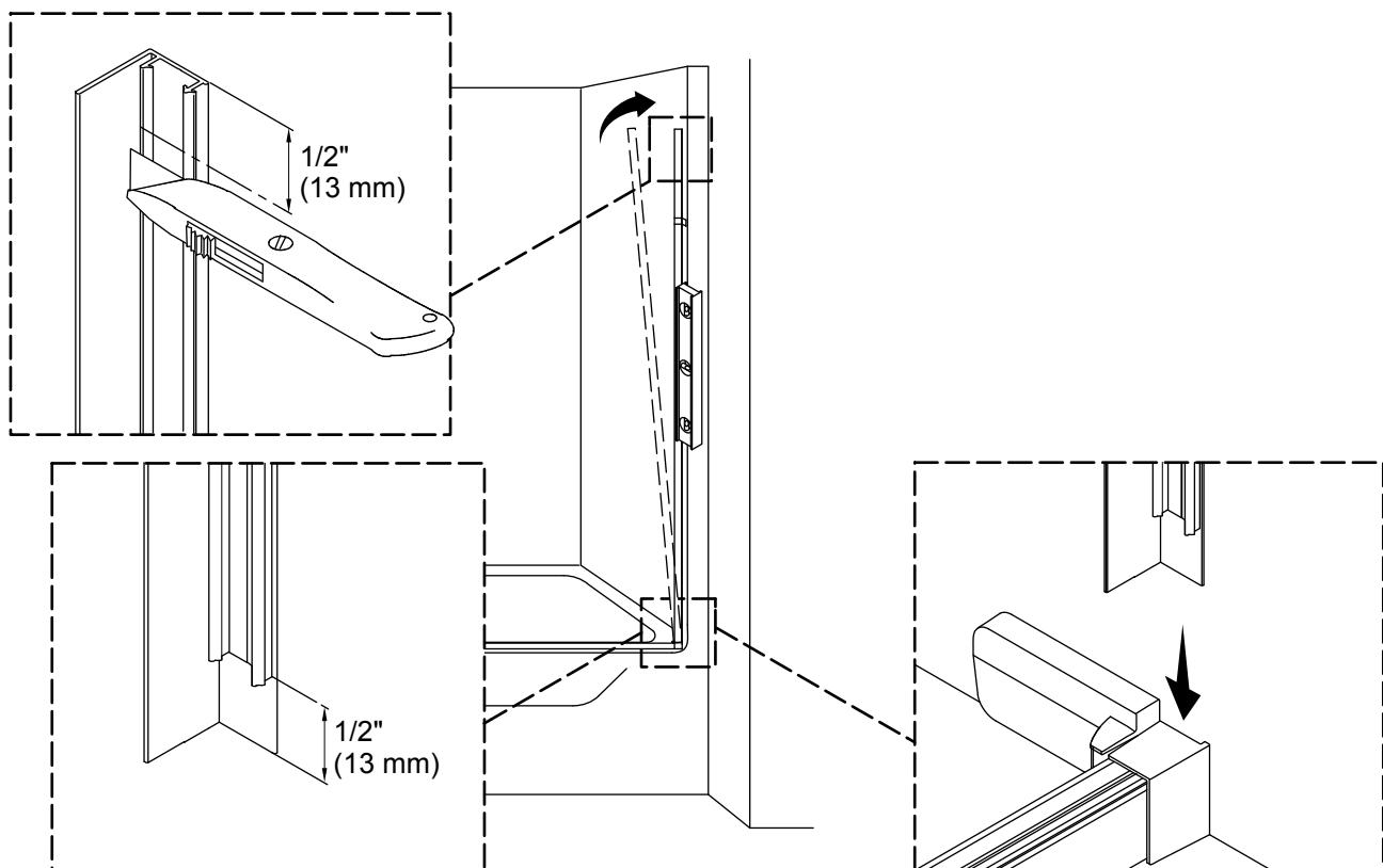
**IMPORTANT!** The wall seal must be level and plumb for proper header installation.
