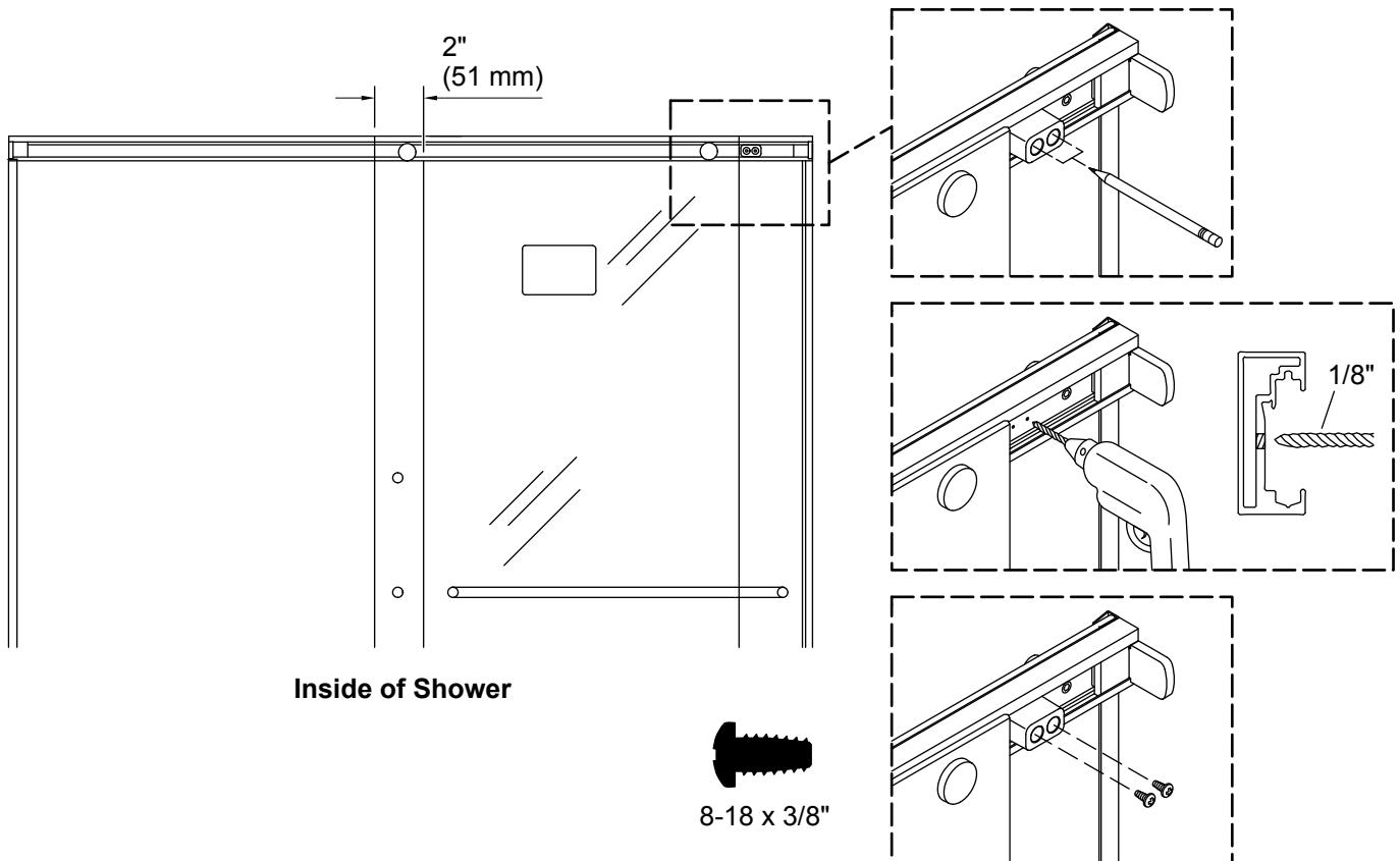
**NOTE:** The top bumper is required for 54" (1372 mm), 66" (1676 mm), and 72" (1829 mm) door sizes. Install the top bumper if supplied. If not supplied, proceed to the next section.
