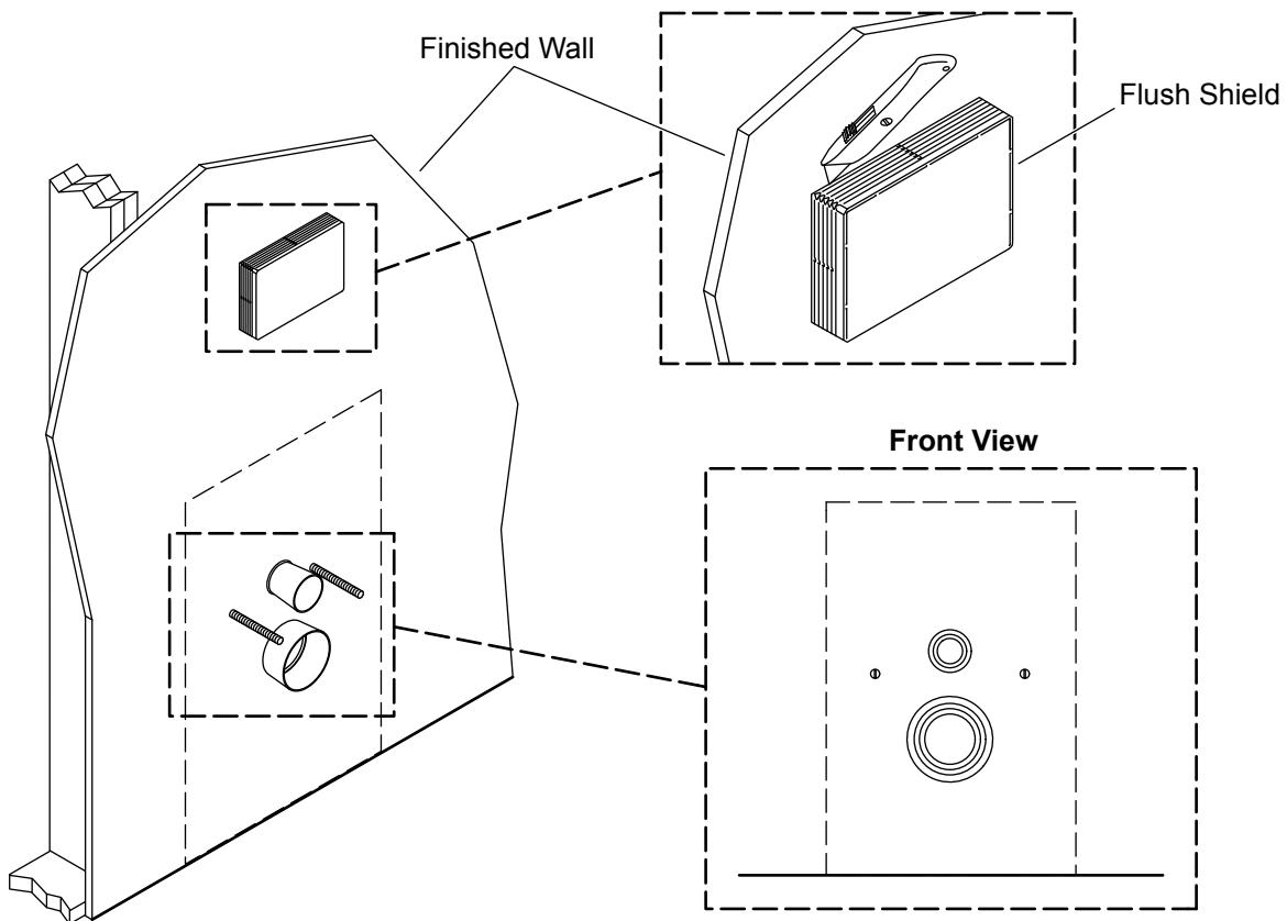
**⚠ CAUTION: Risk of product damage.** Do not puncture the water tank with fasteners. Use the template to determine fastener locations for securing the finished wall. Hang this template on the flush shield to identify the tank location.
