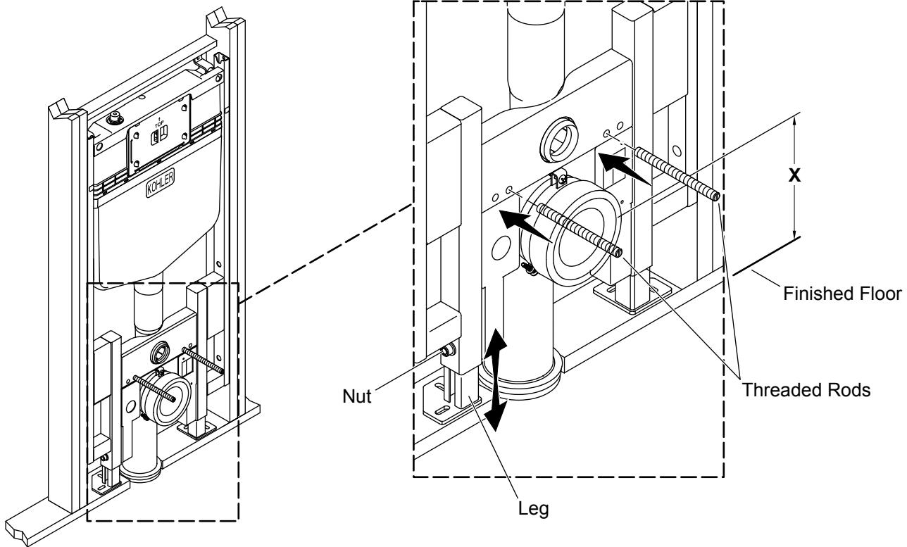
**IMPORTANT!** If the carrier has not been adjusted correctly, the bowl rim height may not be compliant with applicable codes. If the bowl height is not correct, the finished wall will need to be removed to make the required adjustments.
