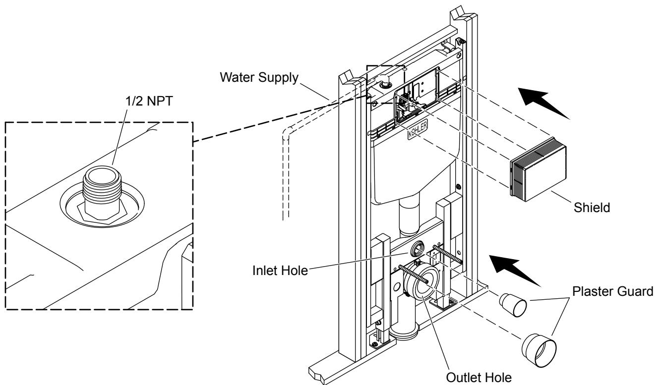
**NOTE:** The tank valve inlet uses 1/2 NPT threads.
