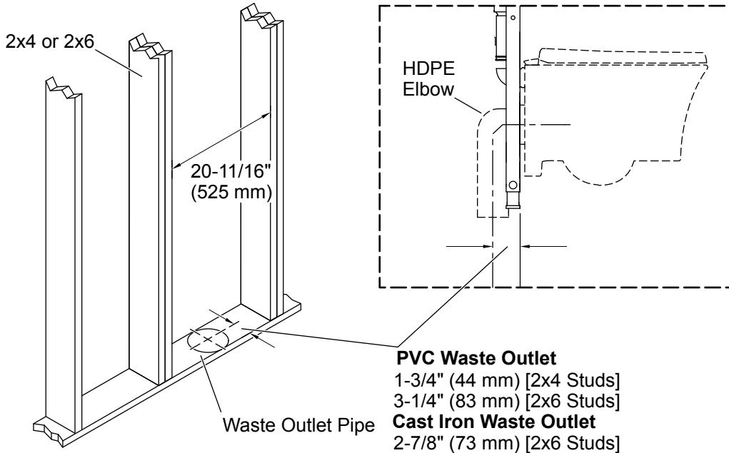
**IMPORTANT!** The waste outlet pipe dimension from the front edge of the framing to the outlet pipe center is critical to this installation. Refer to the illustration above, and see the waste pipe installation options in "Before You Begin" for more details.
