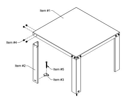
The QUICKSTAND™ #40-S-22- (A or U) stands safely elevates water heaters and other equipment above the floor (650 lbs rating).
