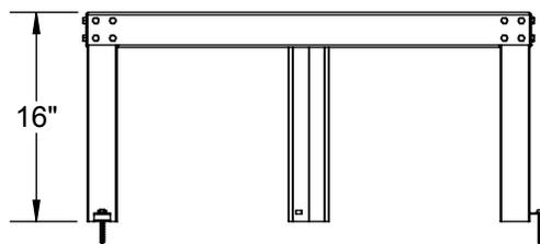
**The QUICKSTAND™ #40-S-34-U stand safely elevates water heaters and other equipment above the floor (2,000 lbs rating).**
