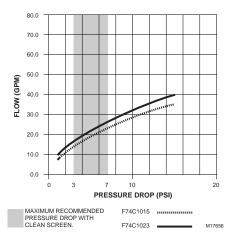
Fig. 2. F74C Pressure drop vs. flow.
