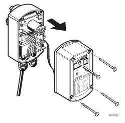
Fig. 11. Removing the MV876 cover.
