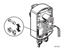
Fig. 13. Replacing the MV876 fuse.
