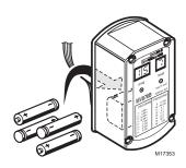
Fig. 12. Installing batteries in the MV876.
