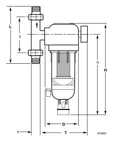
Fig. 1. Dimension drawing of F74C.
