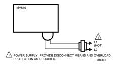
Fig. 14. Wiring diagram for F74C with MV876.
