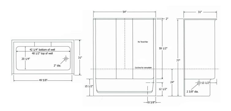
$\textbf{FEATURES} \ \ \text{Dimensional Tolerance} \ \ \textbf{± \%}". \ \ \text{Dimensions needed for site preparation should be measured from the unit. American Bath Group assumes no responsibility for preparatory work.}$
