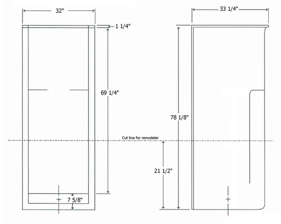
**FEATURES** Dimensional Tolerance  $\pm \frac{3}{16}$ ". Dimensions needed for site preparation should be measured from the unit. American Bath Group assumes no responsibility for preparatory work.
