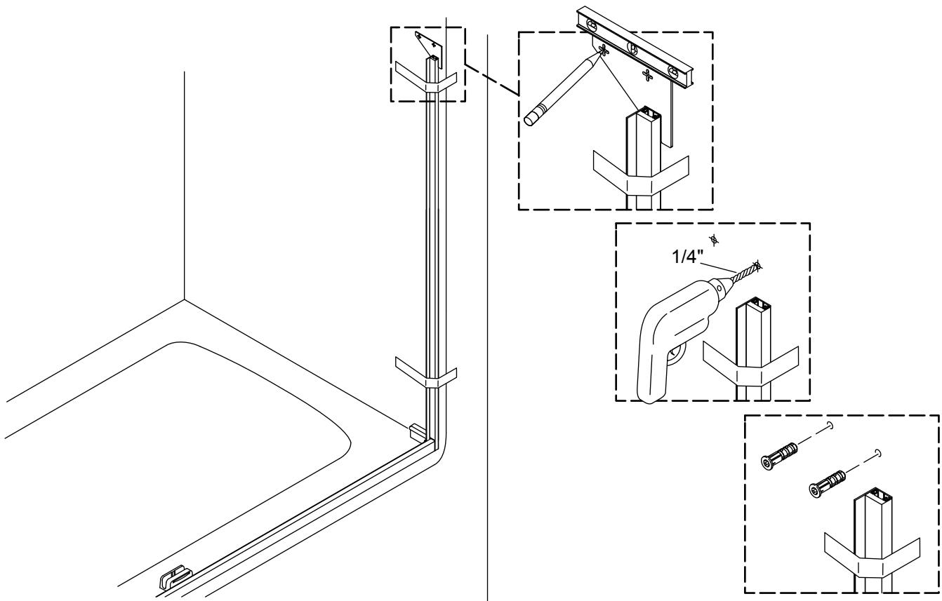
**IMPORTANT!** Hole locations for the wall brackets are critical. Make sure the holes are properly marked and drilled straight into the wall.
