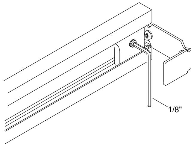
**IMPORTANT!** The header is secured to the brackets in this step so that the door panel may be hung.
