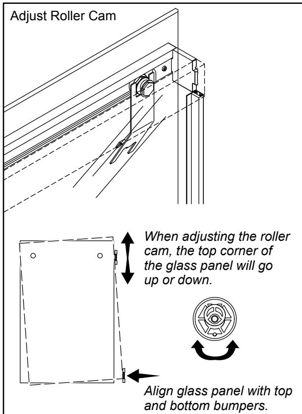
**NOTICE:** The panels may require adjustment to ensure that they touch the top and bottom bumpers in the proper closed position. The inside panel should close on the showerhead side, and the outside panel should close on the opposite side. Adjustment is easiest when done with the panel closed against the correct shower wall.
