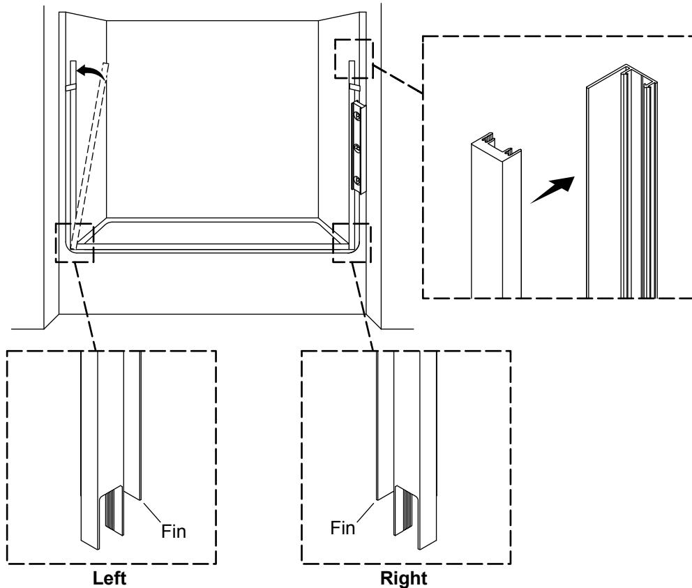
**NOTE:** The flexible fin of the seal is on the inside of the wall jambs.
