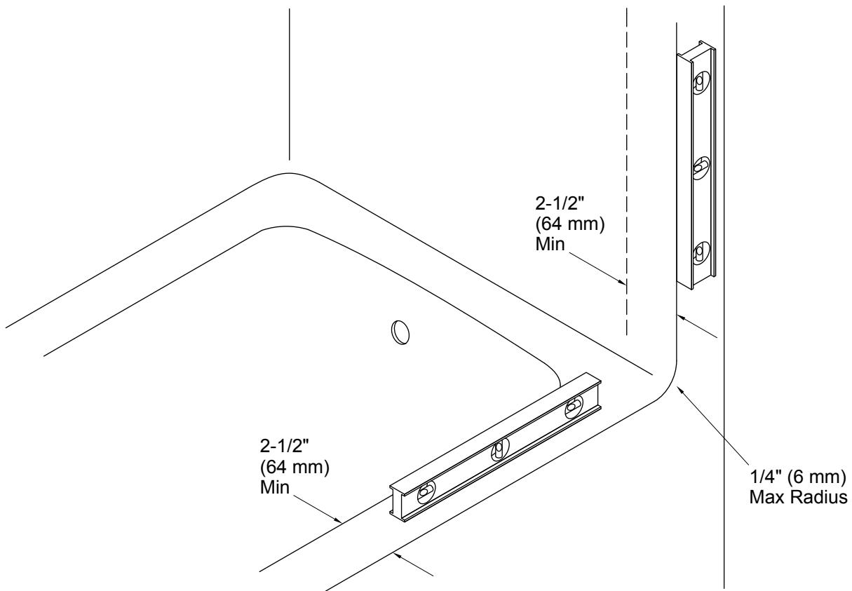
**IMPORTANT!** For proper door alignment and operation, confirm that the shower base/bath ledge and walls meet the following requirements. Do not install the door if these requirements are not met.
