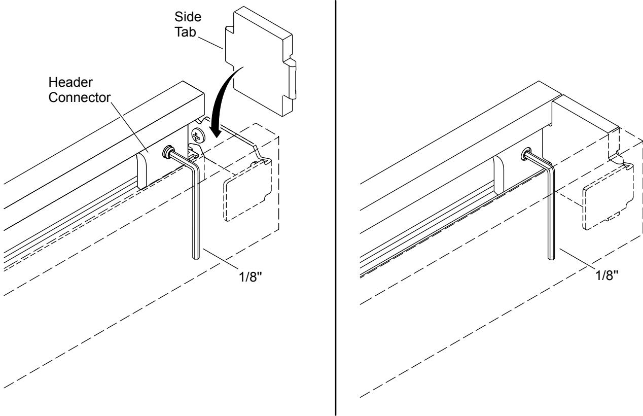
**NOTE:** To ease bumper installation, the header connectors may need to be loosened and temporarily moved away from the bracket.
