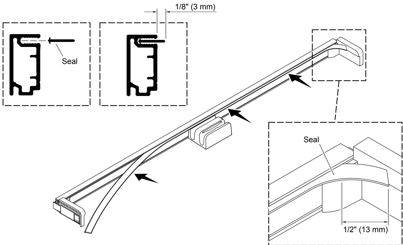
**IMPORTANT!** The seal must be installed with at least  $1/2"$  (13 mm) extending beyond each end of the threshold. The seal will be cut to fit after the threshold has been installed.
