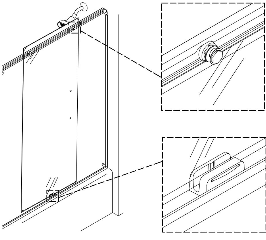
**⚠ CAUTION: Risk of product damage.** Once installed, do not move the panel close to the wall because the top bumpers are not installed at this time.
