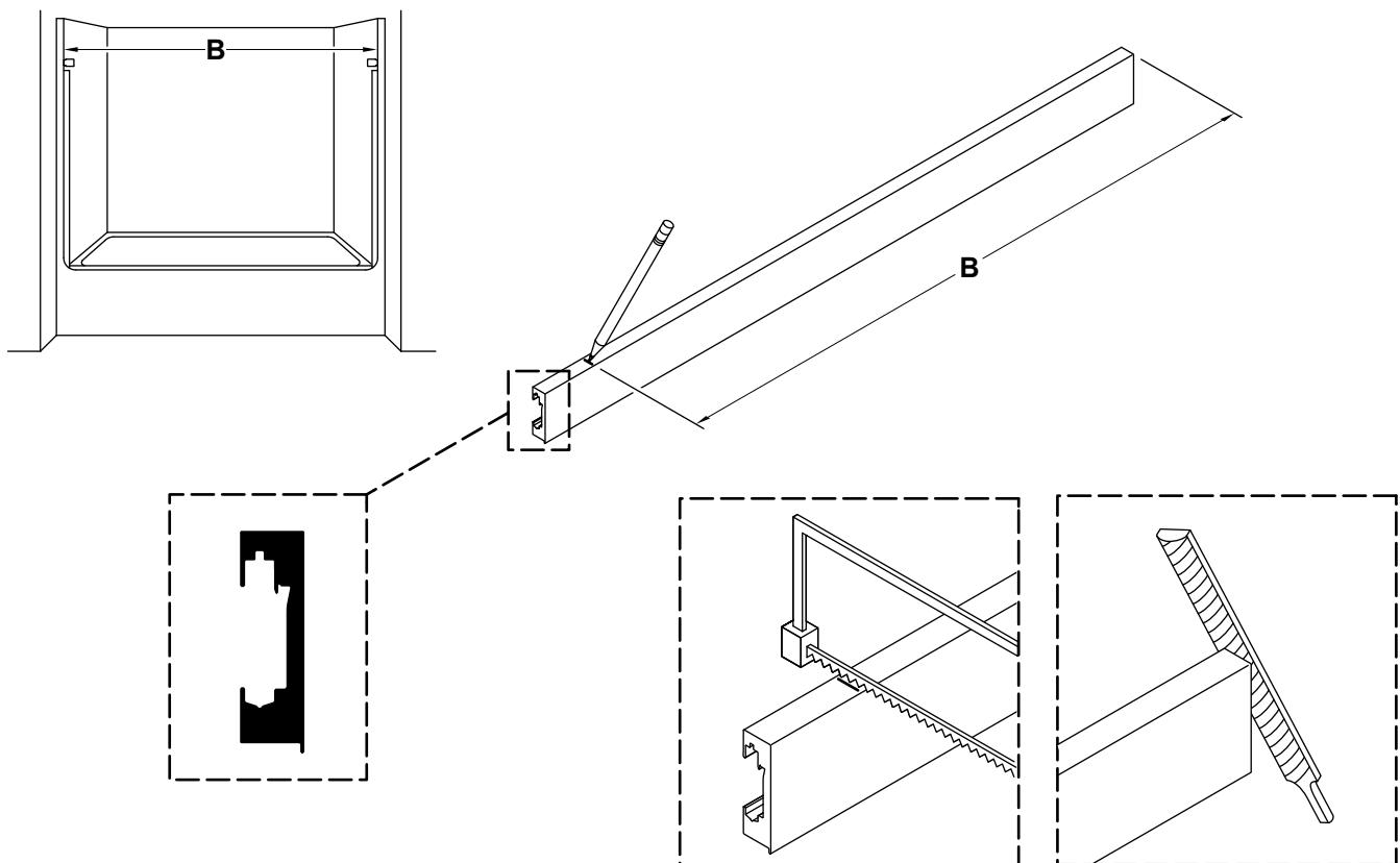
**IMPORTANT!** Confirm your measurements before cutting. Do not cut the header too short.
