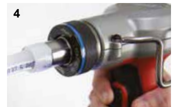
Expansion with Milwaukee M12 ProPEX Expansion Tool
