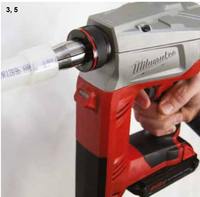
Expansion with Milwaukee M18 ProPEX Expansion Tool
