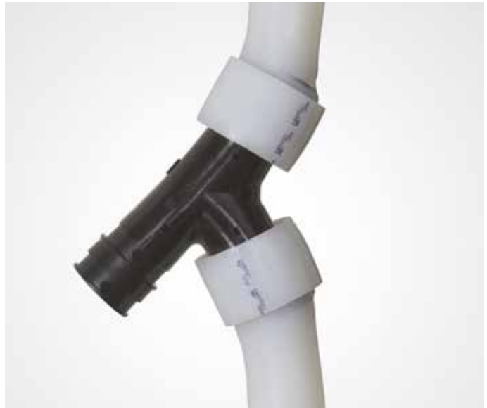
Figure 1-5: At approximately 2,900 lbs. of pull force
