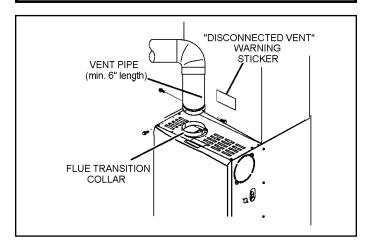
Figure 22. Vent Connection
