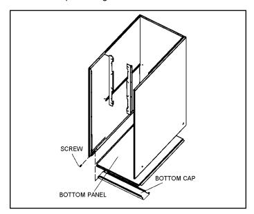
Figure 9. Removing the Bottom Panel
