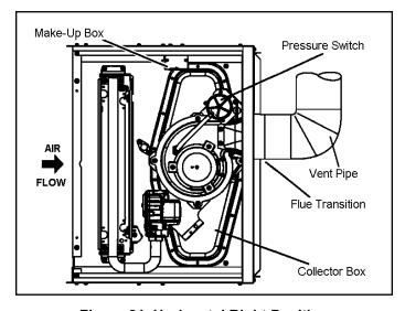
Figure 21. Horizontal Right Position Side Vent Discharge
