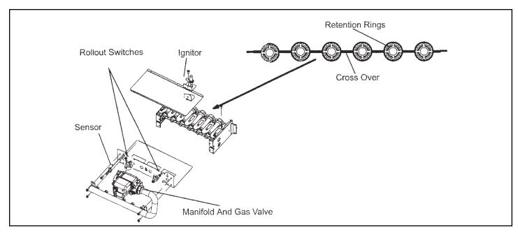
Figure 36. Burner, Combustion Air Inducer Assembly & Heat Exchanger Removal
