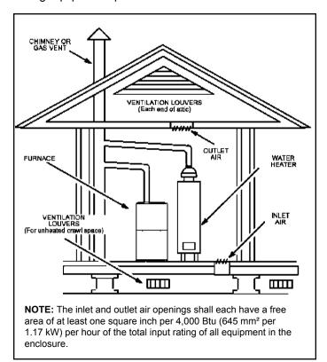
Figure 3. Equipment in Confined Space - All Air from
