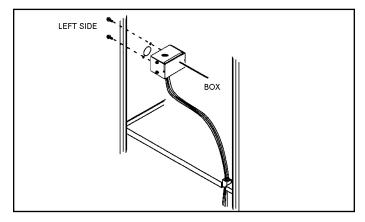
Figure 29. Interior Make-Up Box Installation
