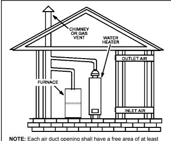
one square inch per 2,000 Btu (645 mm² per .59 kW) per hour of the total input rating of all equipment in the enclosure. If the equipment room is located against an outside wall and the air openings communicate directly with the outdoors, each opening shall have a free area of at least 1 square inch per 4,000 Btu (645 mm² per 1.17 kW) per hour of the total input rating of all other equipment in the enclosure.
