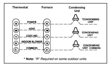
Figure 32. Condensing Unit Thermostat Designations (Refer to Specific Thermostat and Outdoor Unit)
