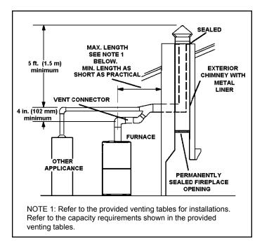
Figure 23. Common Venting Using Metal-Lined Masonry Chimney
