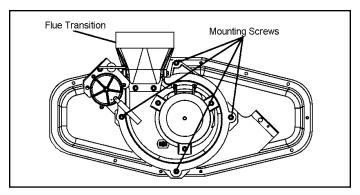
Figure 14. Mounting Screws Location
