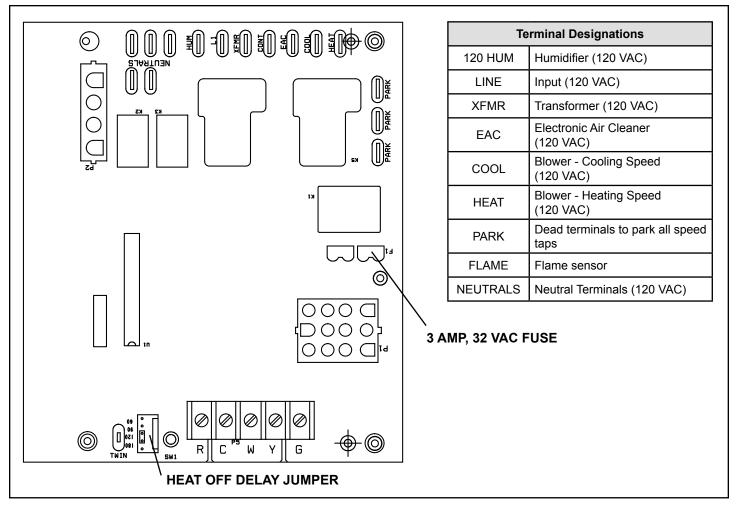
Figure 31. Integrated Control (Automatic Hot Surface Ignition System)
