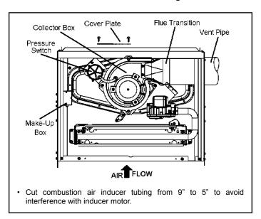
Figure 17. Upflow Position Right Side Vent Discharge
