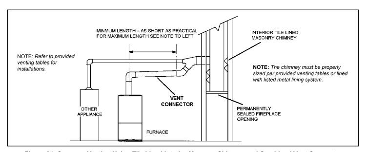
Figure 24. Common Venting Using Tile Lined Interior Masonry Chimney and Combined Vent Connector
