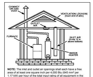
Figure 4. Equipment in Confined Space - All Air from
