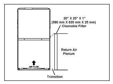
Figure 8. Single Side Return Air (with transition and filter)
