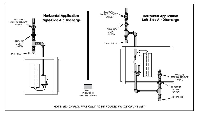
Figure 25. Possible Gas Piping Configurations - Horizontal Applications
