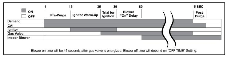
Figure 34. Integrated Ignition Control
