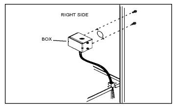
Figure 28. Interior Make-Up Box Installation
