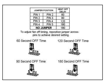
Figure 35. Heat Fan Off Time in Seconds
