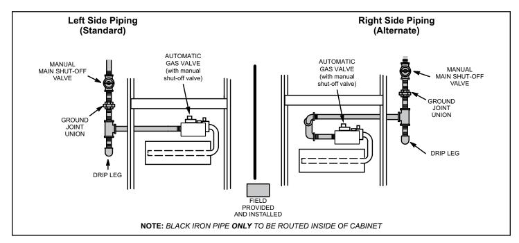
Figure 27. Possible Gas Piping Configurations - Upflow Applications
