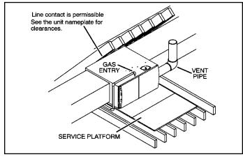
Figure 13. Horizontal Application Unit installed on Platform
