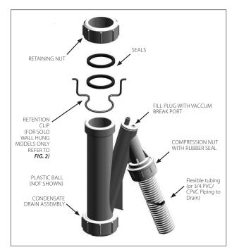
Fig. 1 - Condensate Drain Assembly
