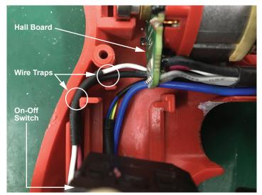
Push black and white wires completly down in wire traps. Route blue and yellow wires behind on-off switch.
