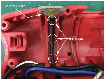
Tuck Shutter Board squarely and firmly in slotted recess of housing support. Push wires completely down in wire traps.
