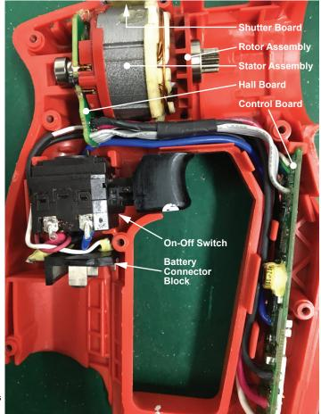
Be sure all elements of the electronics assembly are firmly seated in the support housing. Be sure all wires are pushed completely down in wire traps and channels. Make sure there is no interference prior to installing the housing cover.
