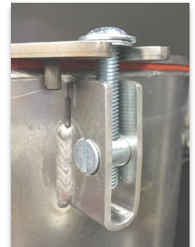
New 399 heat exchanger bolt design
