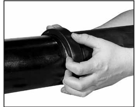
**3 ALIGNMENT**— After aligning the two pipe ends together, pull the gasket into position, centering it between the grooves on each pipe. The gasket should not extend into the groove on either pipe.
